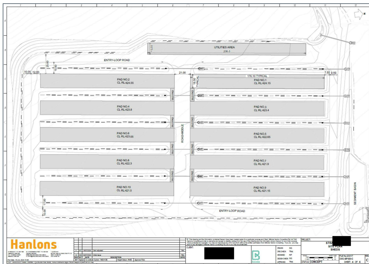
Figure 10: Modified Shed Pads (Hanlons, 2024)
